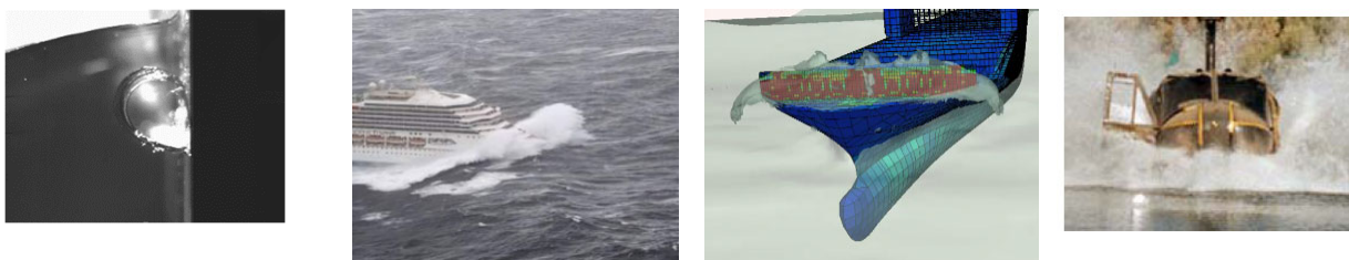
Figure 59: Practical hydrodynamic impact situations (from left to right: sloshing, slamming, green water, ditching)
